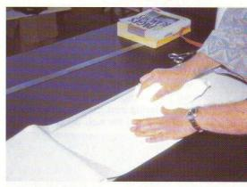
To avoid any creases that would be tragic for the result, progress gradually towards the wing tip sticking the vinyl to the leading and trailing edges (LE &TE) only after the point where you have stuck the vinyl to the middle of the chord. If you progress too rapidly on the LE and TE you are certain to have terrible creases.
