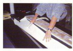
Vacuum clean the two faces of the vinyl panel before spreading it over the under surface of the wing (still with the backing attached).
