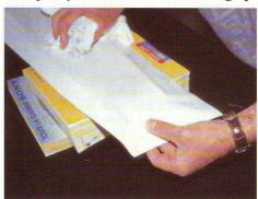
Immobilise the wing on the worktable with something heavy: Then with a hairdryer in one hand, carefully warm the film whilst pulling it with the other hand. You will see that the vinyl becomes soft and can easily follow the wing tip shape.
