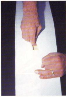
When done you can carefully sandpaper the join line to reduce it an absolute minimum before starting to cover the upper surface.
