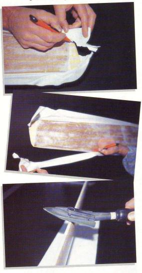
To fold back and stick the vinyl against the root and servo boxes first cut the vinyl with a small margin (3 to 4 mm), then vigorously rub the vinyl on the edge (with the rag or directly with the finger), with heat it will almost mould around any angle.
