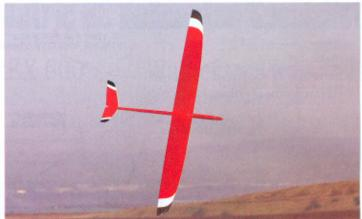
Modern slope racing gliders are designed with the exploitation of camber changing flaps in mind.
