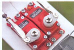
Switching between flight modes for camber and reflex, offsets the neutral position of the trailing edge of the wing. Alternative differential settings will be needed in each flight model to overcome this.
