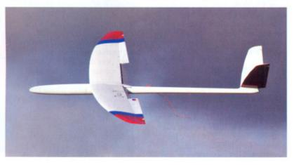
Crow braking provides a predictable and efficient way of slowing down your slippery glider for landing. Get your mixes right and this method makes it easy to pick your spot for touching down.
